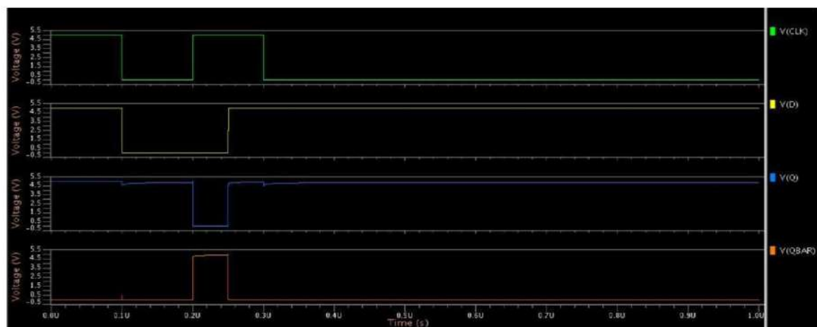
Figure 12: Shows Results of D flip flop using transmission gate logic
